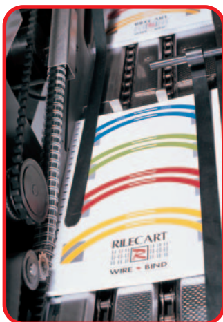
Wire feeding system.
