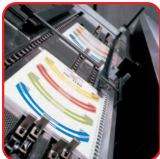
The wire out of tunnel reaches the binding area.
